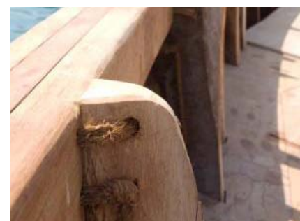
■ No nails used to secure any part of the ship
